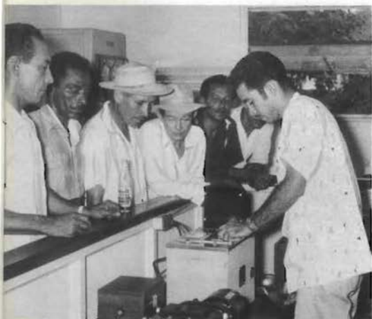
(Left) The laboratory determines the moisture content of each bag of corn by electronic measurement of its resistance to a current of electricity. (Right) Carrying dockets giving the weight of his corn and its moisture content, the campesino is paid for his consignment by the busy IFE cashier.
